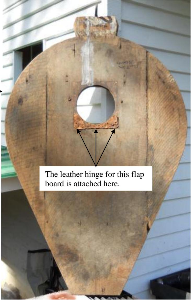
The leather hinge for this flap board is attached here.
