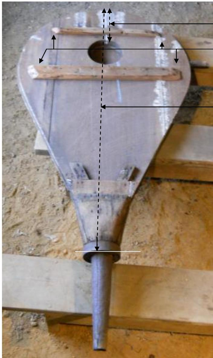
It's 11 & 1/8" from top on the Center Board to the top of the hole. The Lower Board hole is directly under this hole.
